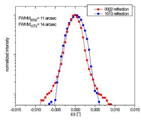
Fig. 3: Rocking curves (semi-logarithmic scale) measured with 4-bounce Ge-220 monochromator and open detector aperture over the full as-grown (000-1) facet area of a typical AIN crystal in the 0002 and 10-13 reflections
