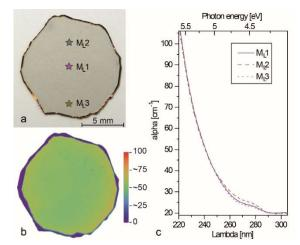
Fig. 2: (a) Optical image of a c-plane AIN wafer ( $\emptyset \sim 11 \text{ mm}$ ) with measuring spots; (b) transmittance of this wafer at 254 nm (wafer thickness = 140 µm); (c) absorption spectra at the measuring spots. Except for the outermost rim, the entire AIN wafer shows  $\alpha_{265 \text{ nm}} = 25-28 \text{ cm}^{-1}$
